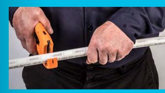
Step 1 Cut the desired length of pipe. • Square cut, perpendicular to length of tubing
